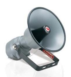
SSTX3-MV is an explosion-proof electronic siren capable of producing three high decibel tones from the same unit. The integrated circuitry is contained in a rugged die-cast aluminum housing. The unique threaded rear access cover eliminates traditional time consuming bolting patterns. The access cover is also equipped with a braided cable lanyard securing it to the housing whenever the cover is open for installation or maintenance.
